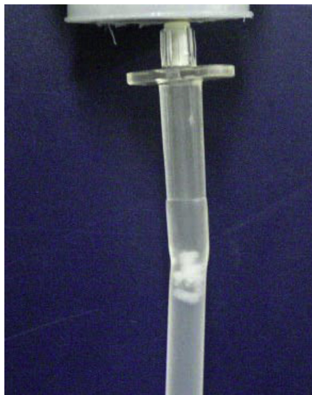
Fig. 1. Photograph of aggregation substances in suspension with Formulation #3 and Hartmann's solution pH 8.
